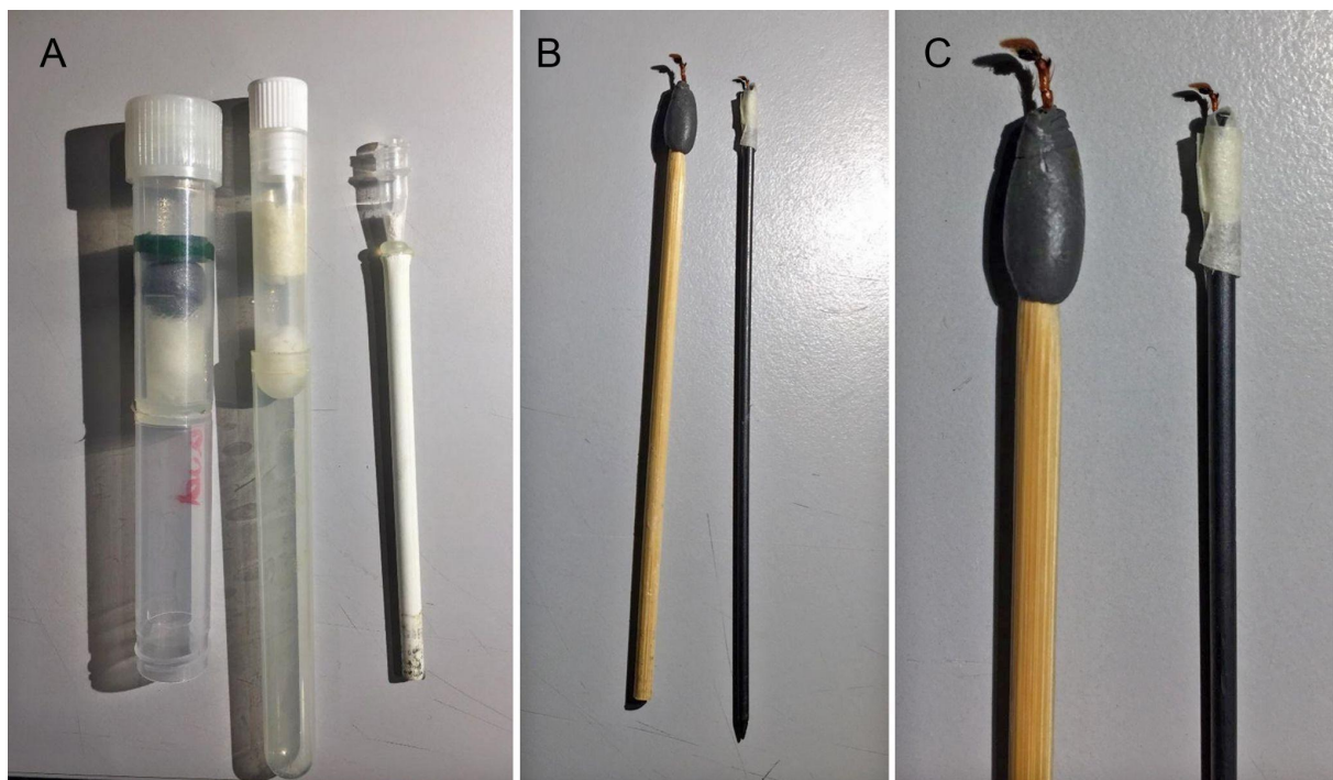
Figure 35. The results are however much better when the palp is air-dried (still after staining) and scanned freely. Dried palp is easier to prepare, gently fixed on top of a wood or carbon stick, using plasticine or low tack tape (see Figure 35-C). The sample can be rehydrated using a wetting agent as described in Jocqué (2008) and Baccaloni (2012). For example, a comparison of results without and with LUGOL treatments and scanned in aqueous solution or in the air can be seen in Figure 34.
