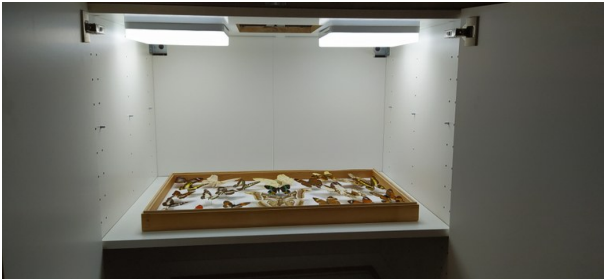
Figure 18: Setup for the digitization of the complete insects boxes using two top led panels
