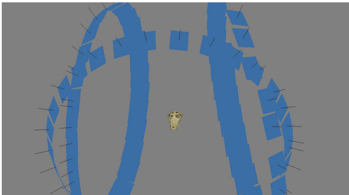
Figure 23: Aligned 108 pictures (3 rotations) used to create the 3D model with the SfM Agisoft Photoscan
