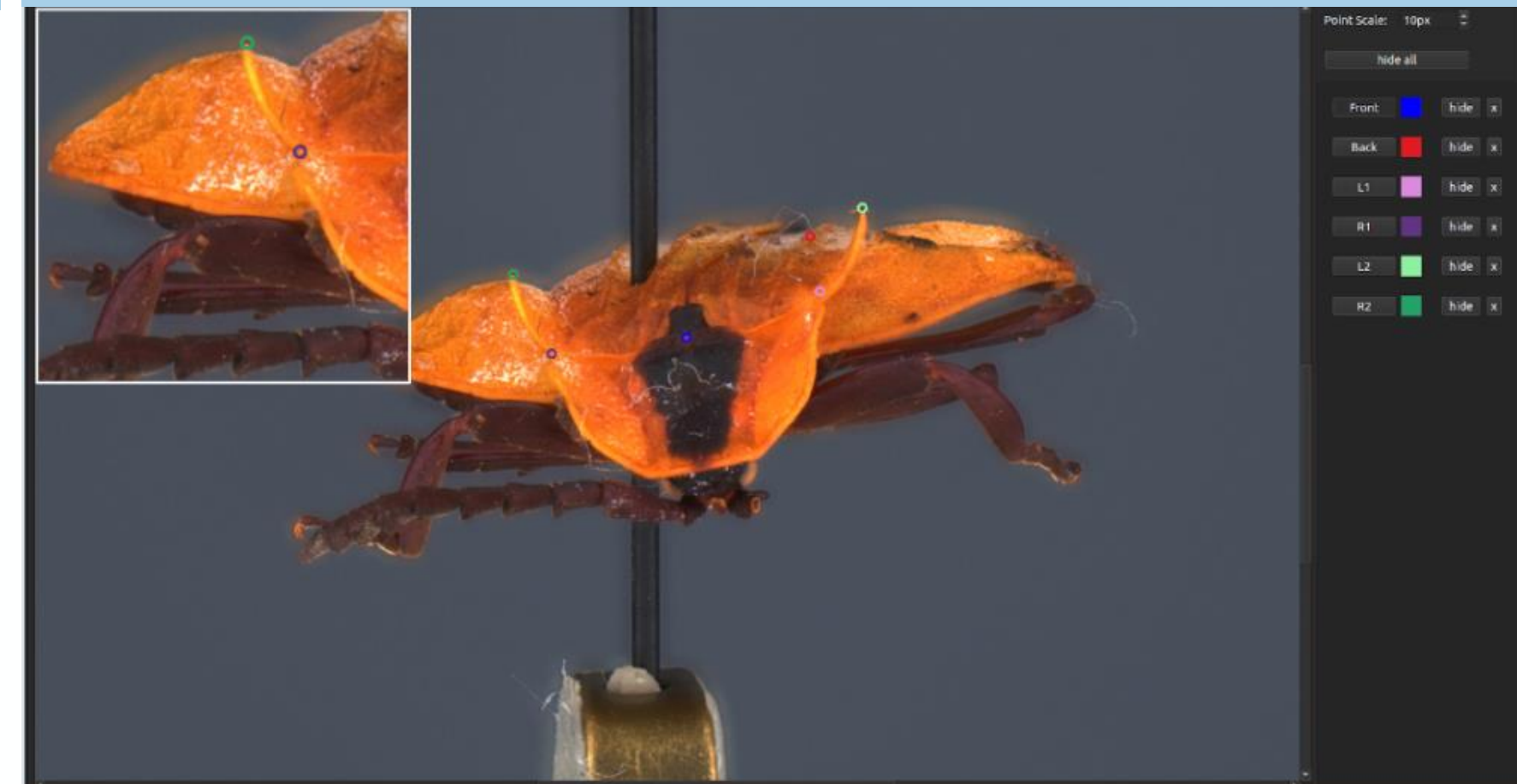
3D landmarks on 2D stacked images using ORTHANC as server and Sphaeroptica as viewer
